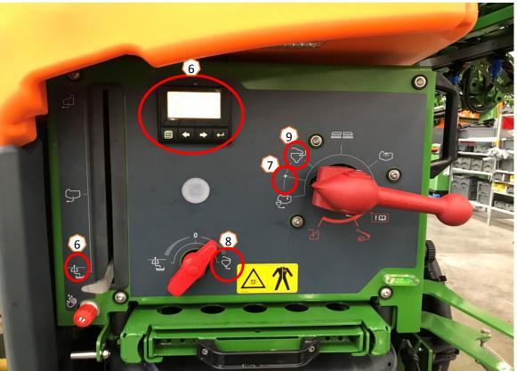
After the sprayer has been filled and the crop protection products have been flushing in, the pressure tap must be switched to "Spraying". (1)
